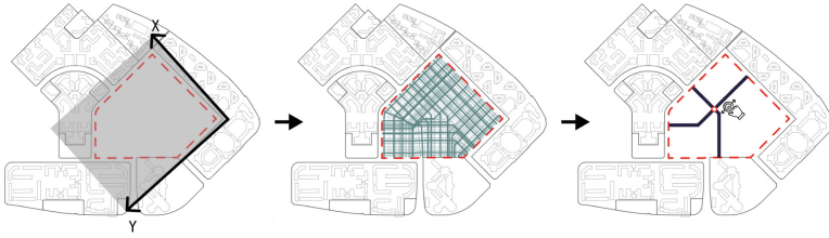
Fig. 1. Progressive steps to generate urban fabric: 1) Site selection (red dashed line) and computation of best-fit orientation plane (grey plane); 2) Generation of all streamlines (teal); 3) Selection of streamline pair to subdivide plot.
